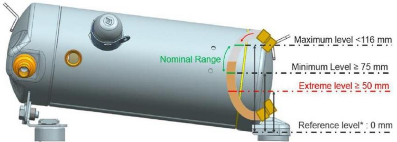
Figure 12 Acceptable Oil Level
