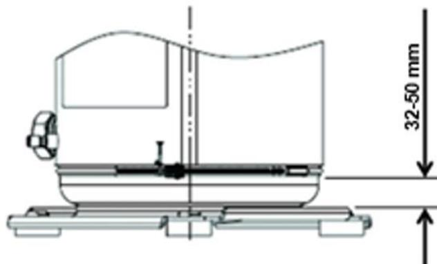
Connect the heater so the connection point straddles the compressor weld seam
