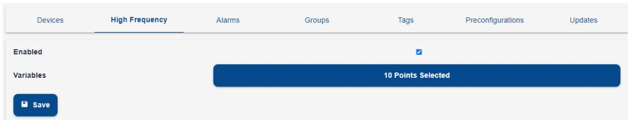
The screenshot shows the XWEB PRO Monitoring System interface. The top navigation bar includes 'Devices', 'High Frequency' (which is the active tab), 'Alarms', 'Groups', 'Tags', 'Preconfigurations', and 'Updates'. Below the navigation is a search bar with the placeholder 'Enabled'. The main content area is titled 'Variables' and shows a list of selected points. A blue bar at the top of the list indicates '10 Points Selected'. At the bottom left is a 'Save' button.
