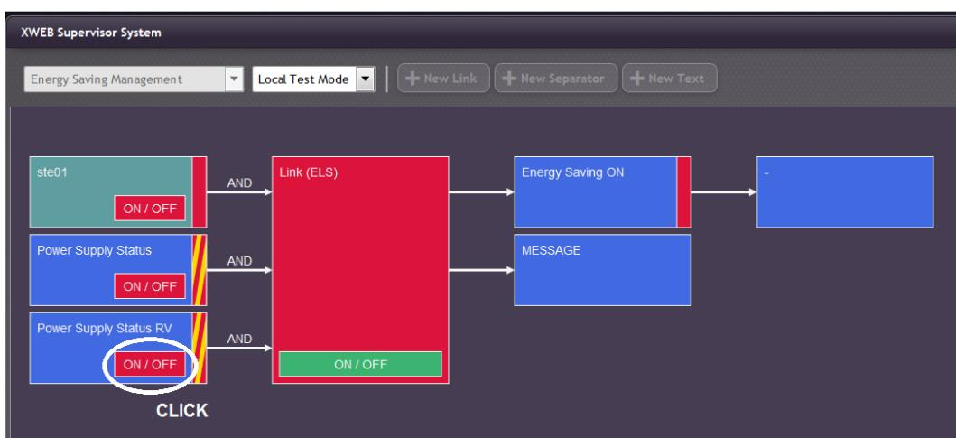
In the above image, we clicked on the SDC block when in status DIS: block enabling activates block ELS which then turns red. And the ODC block sends a false command.
