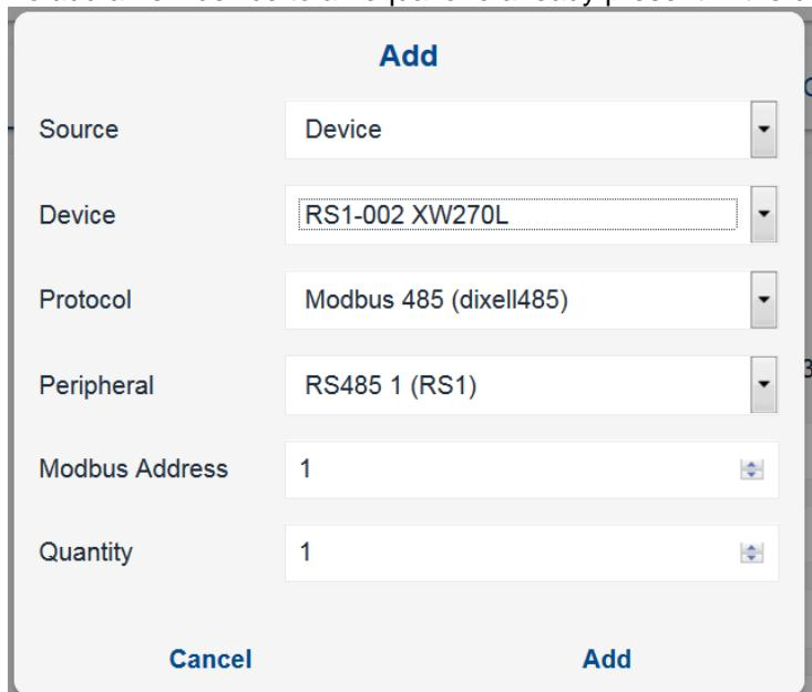
The screenshot shows the 'Add' dialog box. The 'Source' dropdown is set to 'Device', and the 'Device' input field contains 'RS1-002 XW270L'. The 'Protocol' is set to 'Modbus 485 (dixell485)', 'Peripheral' to 'RS485 1 (RS1)', 'Modbus Address' to '1', and 'Quantity' to '1'. At the bottom are 'Cancel' and 'Add' buttons.
