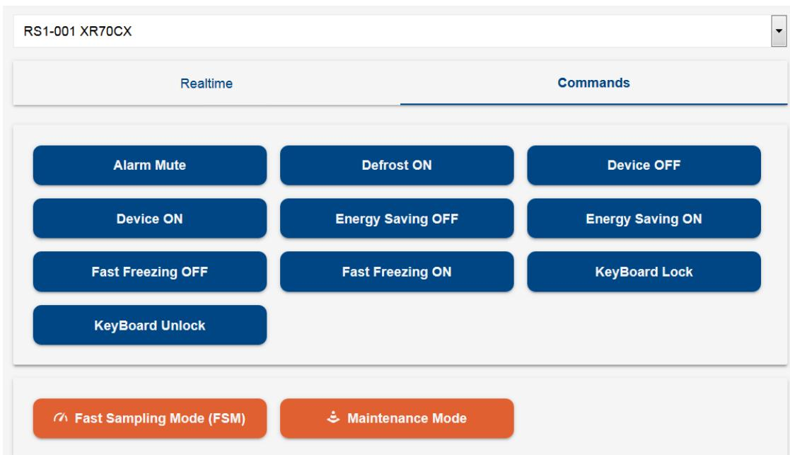
for the selected tool it shows, with blue keys, the available commands that can be sent to the device itself. The list of available commands depends on the type of tool.
