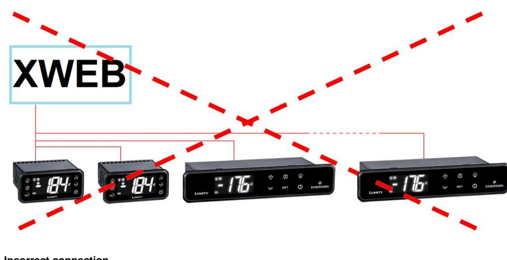
On the same line, each controller is normally programmed with its own unique serial address, through the Adr parameter. Refer to the installation manual of the instrument itself for the access and modification procedure. To obtain a simple description of the categories to which they belong, divide the programming of the addresses progressively. Some special cases are listed on the following pages.
