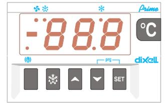
**SET:** To display target set point; in programming mode it selects a parameter or confirm an operation.
