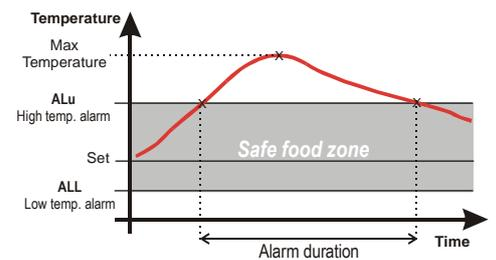
**5.1 HOW TO SEE THE ALARM DURATION AND MAX (MIN) TEMPERATURE**
