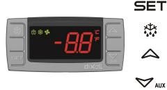
To display target set point, in programming mode it selects a parameter or confirm an operation
